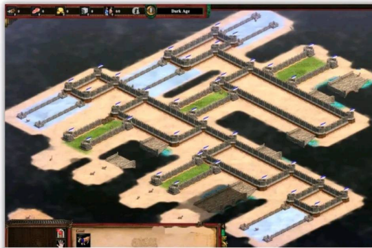
Figure 1: NAND gate in AoE II's editor, designed to show its internal workings—simpler implementations are possible. Every bit is represented by two rails (grass for 0, a bridge for 1). Only one rail is active at a time, with a goat acting as the signal carrier. When the gate fires, the bit-goats are removed and a new bit-goat is placed in its respective output rail. To avoid race conditions, 'gate ready' rails (ice) are set, with a signal-goat in the rail closest to the gate indicating that it can start the calculation.
